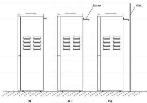
2. Install a bracket where you have removed the screw already, fix the bracket tightening this removed screw on the right location (Picture 2).
